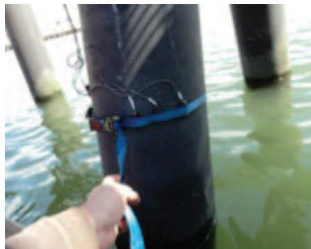
NDT Corporation testing piles to determine pile lengths and depth of embedment.
