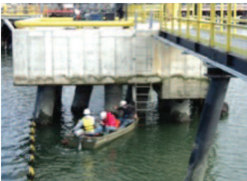
NDT Corporation testing piles to determine pile lengths and depth of embedment.
