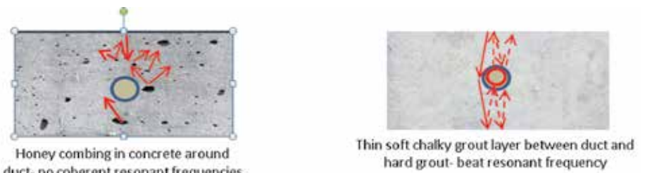
Fig. 6—Diffracted sonic wave paths.
