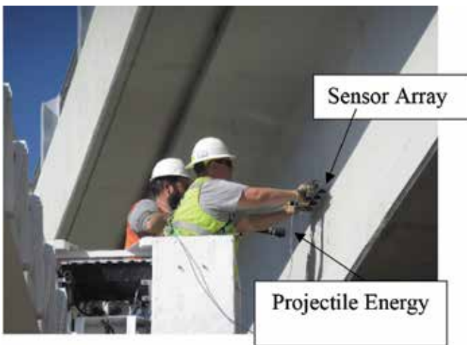
Fig. 3—Impact echo testing.
