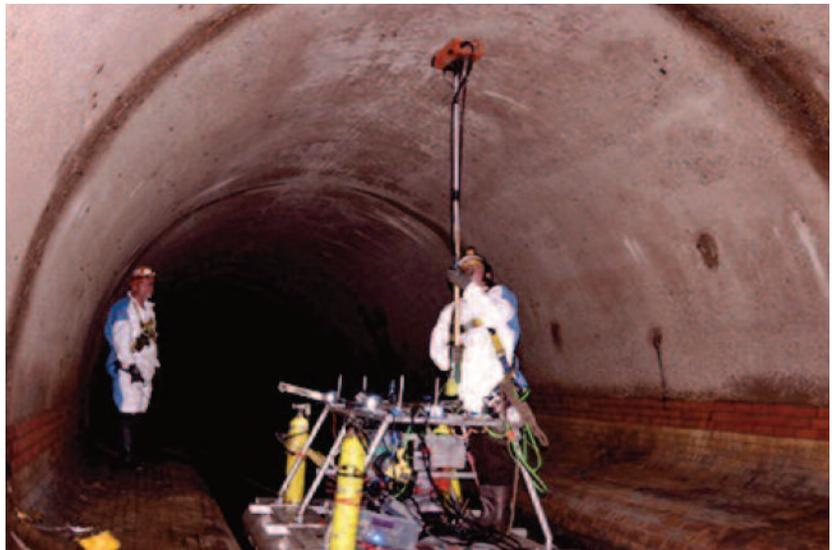
Pipe Penetrating Radar Team Assessing Concrete Liner.
