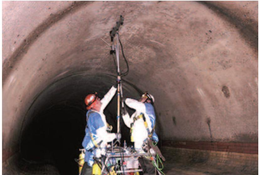
Sonic/Ultrasonic System Used to Determine Concrete Liner Mechanical Integrity.
